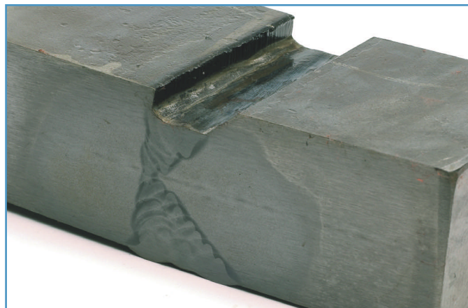
A multi-pass weld sample (some weldments require as many as 70 passes), performed via automation.
